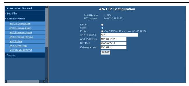
At the top the screen shows the serial number and MAC address of the AN-X being configured. Check either DHCP or Static.
