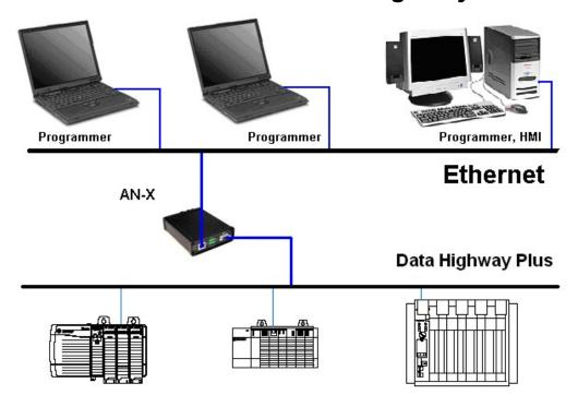
The AN-X4-AB-DHRIO module running Data Highway Plus (DH+) firmware connects a computer or other device on Ethernet to an Allen-Bradley Data Highway Plus network.
