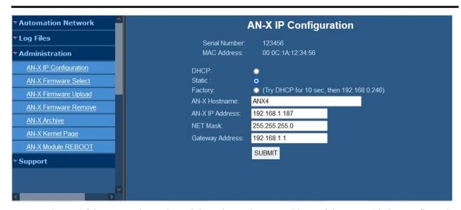
The top of the screen shows the serial number and MAC Address of the AN-X4 being configured.
